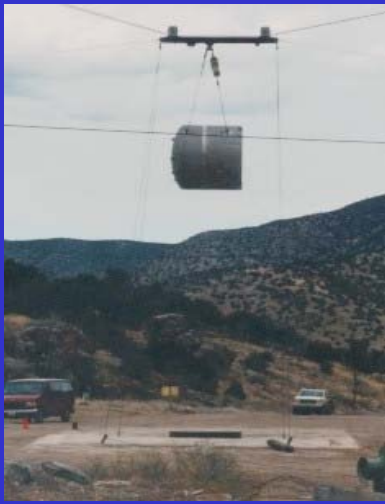
30 foot drop onto essentially unyielding surface
