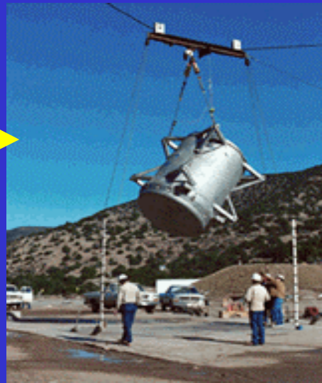
40 inch drop onto 6 inch steel spike
